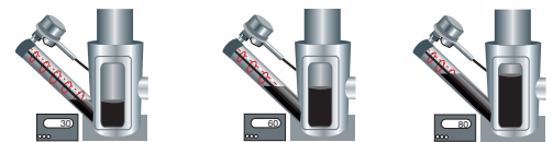
The diagrams are examples of a fluid level inside the nipple, represented by a reading from 1-100 that is displayed at the rig floor.
