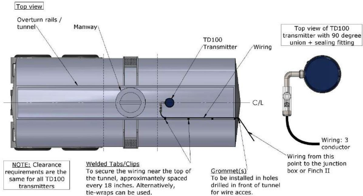
Figure 30 TD100 System Mount - Top View
