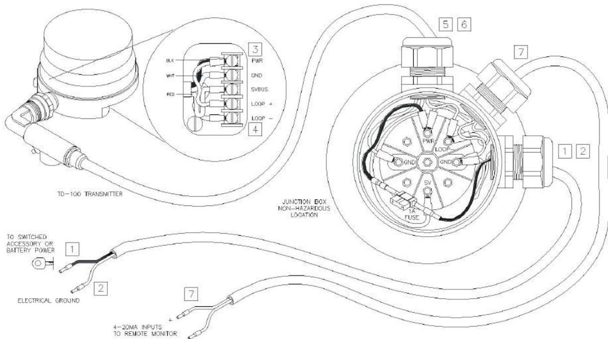
Figure 43 Current Loop Wiring Diagram
