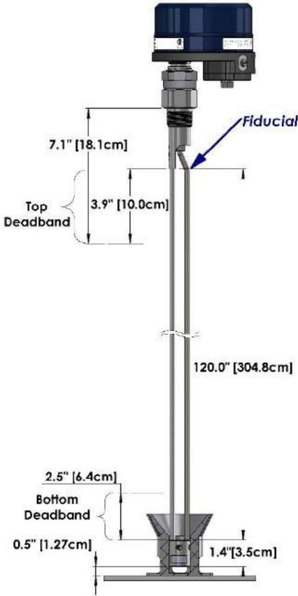
Figure 13 Deadband Areas – Dual Rod Performance Detection Mode
