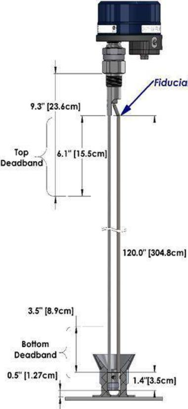
Figure 14 Deadband Areas – Dual Rod Standard Detection Mode
