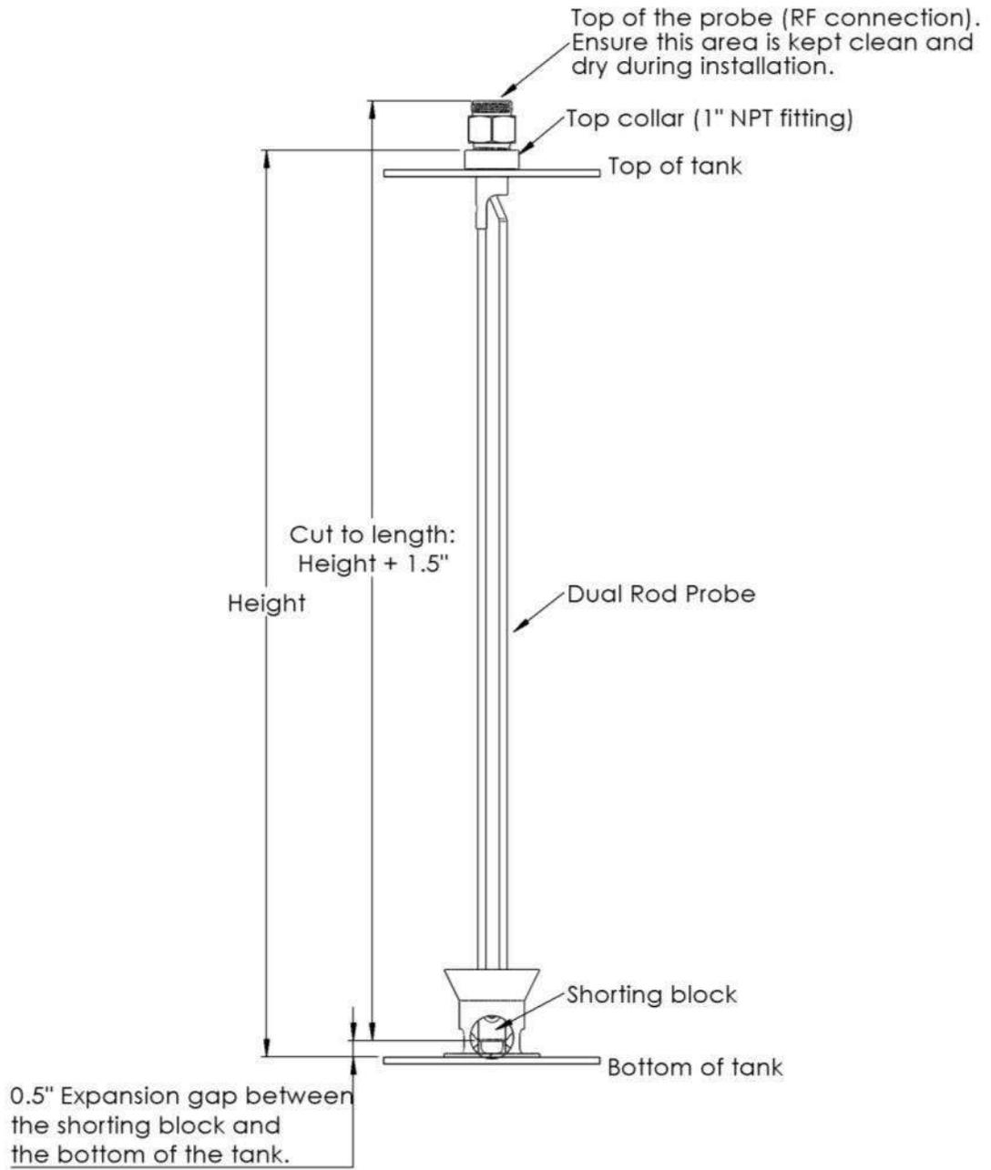
Figure 35 Probe Measurement
