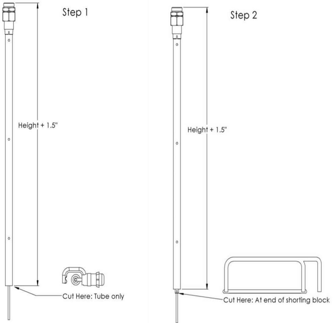
Figure 38 Cutting the Coax Probe
