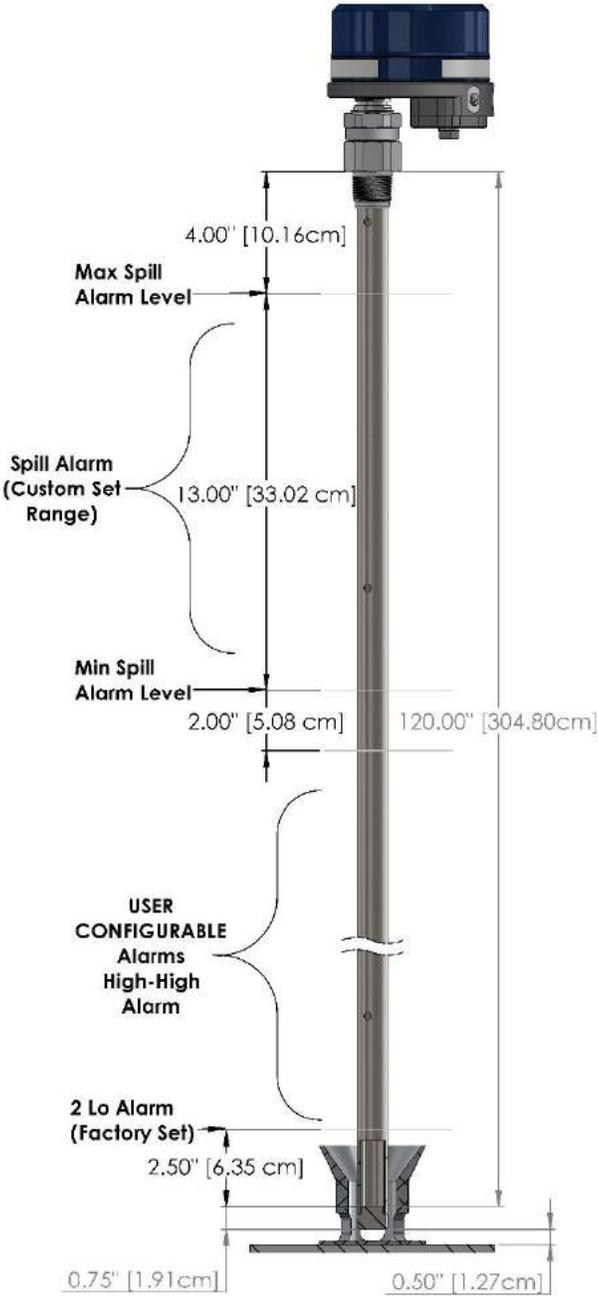
Figure 21 Alarm Points – Coax Performance Detection Mode
