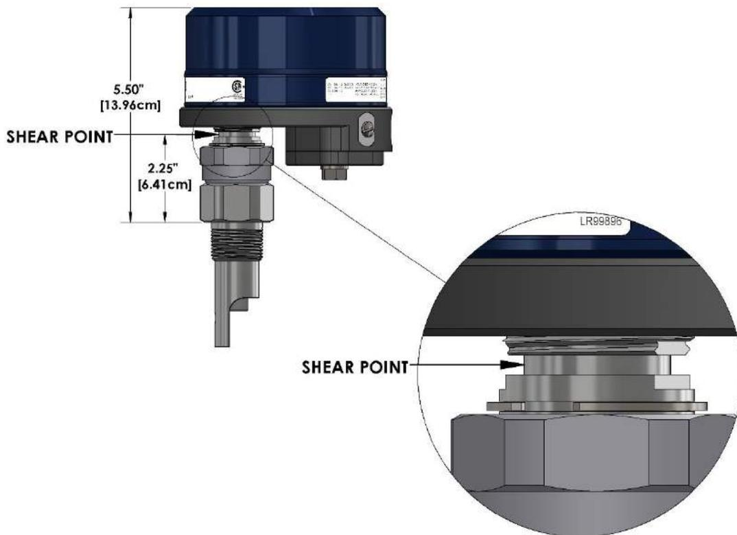
Figure 12 Transmitter Head Shear Point
