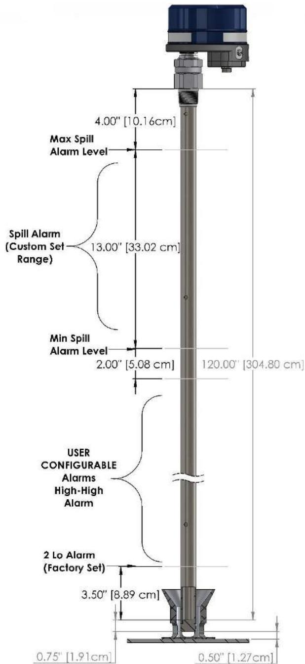
Figure 20 Alarm Points – Coax Standard Detection Mode
