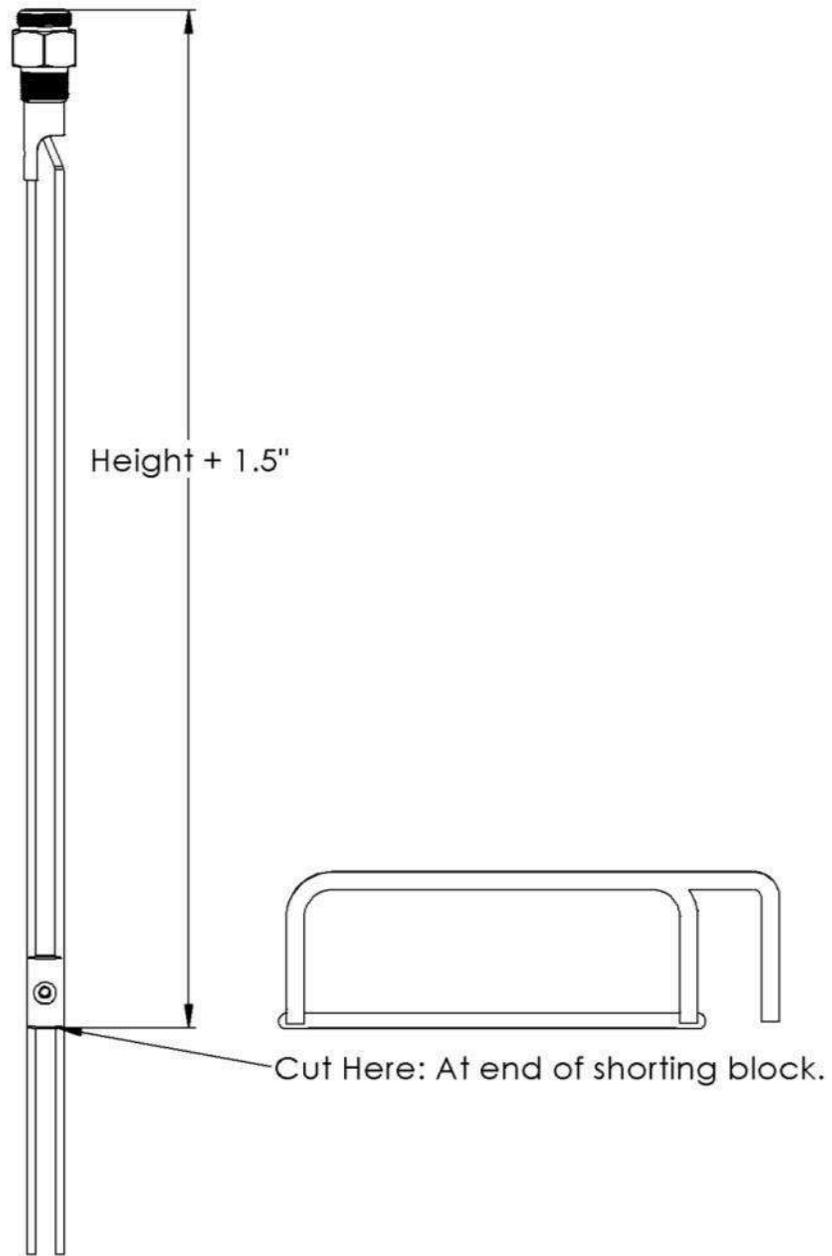
Figure 36 Cutting the Dual Rod Probe
