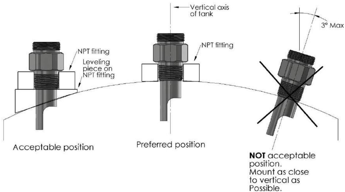
Figure 32 Curved Surface Fitting Mount
