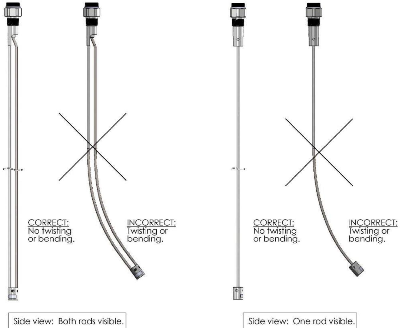
Figure 39 Probe Installation
