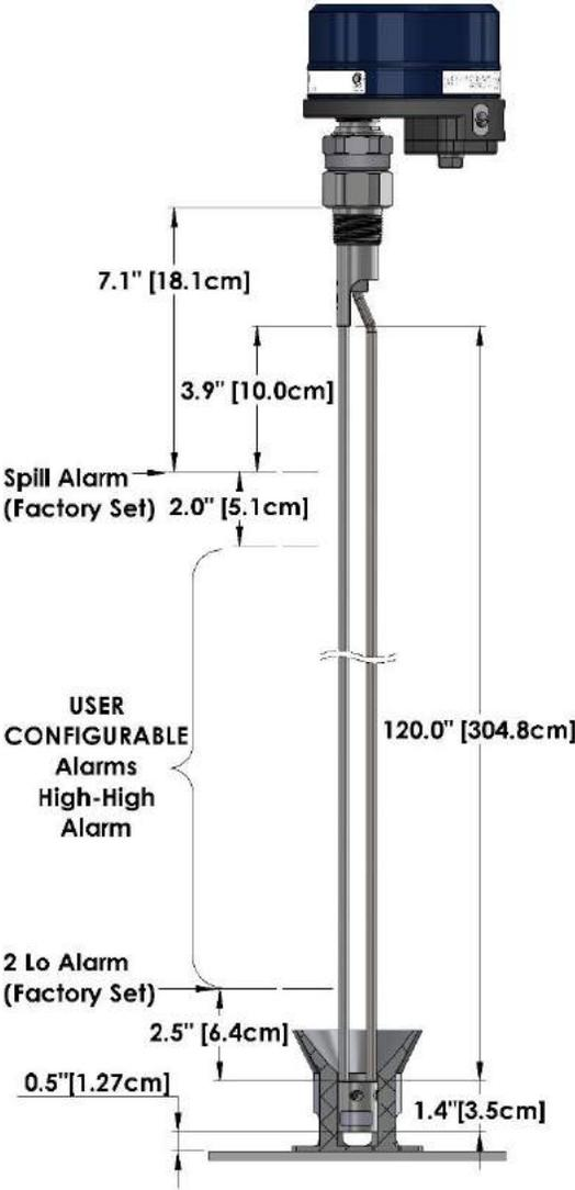
Figure 19 Alarm Points – Dual Rod Performance Detection Mode
