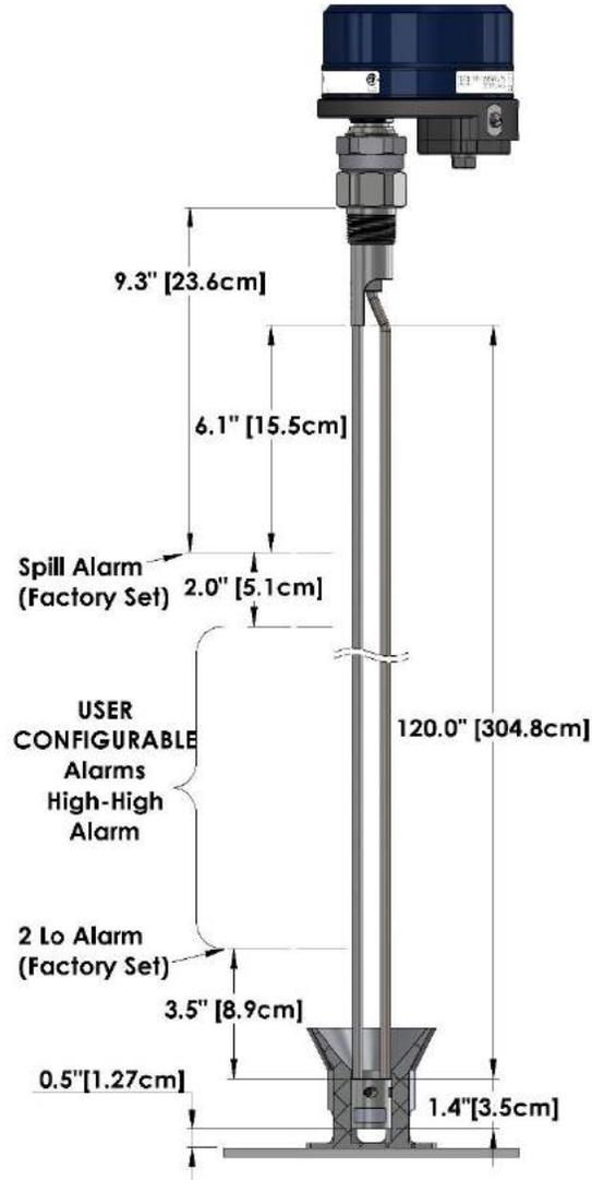
Figure 18 Alarm Points – Dual Rod Standard Detection Mode
